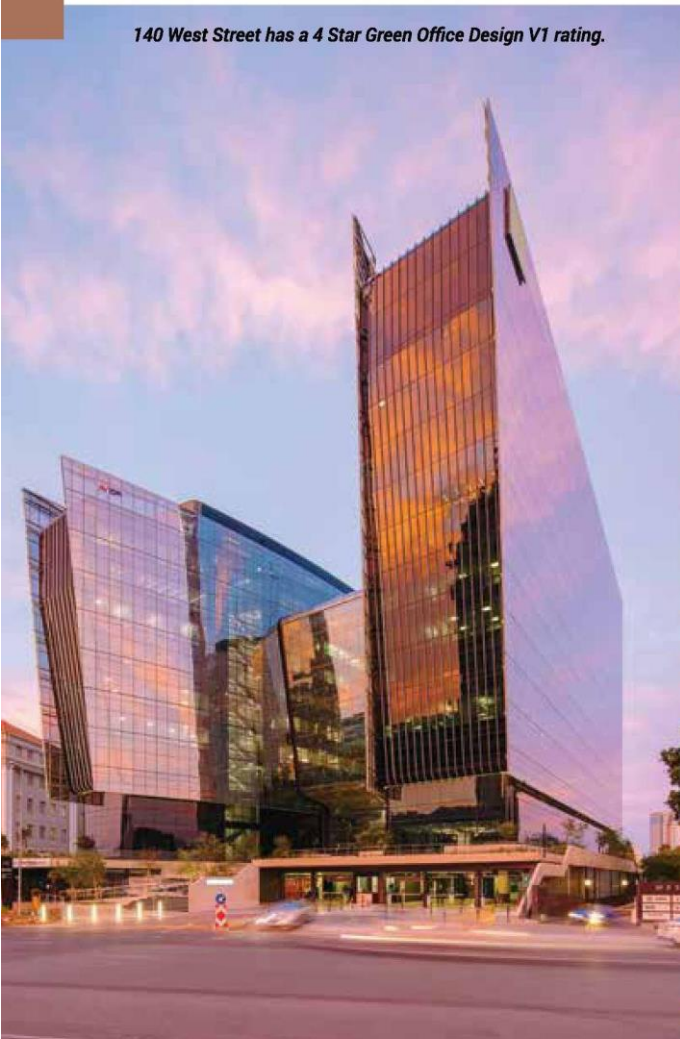
An angled, curved-glass atrium enclosure connects the two towers.
